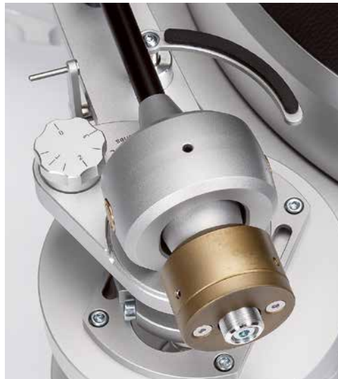
An additional weighting layer can be screwed onto the brass counterweight. The antiskating works by means of a spring balancer.
